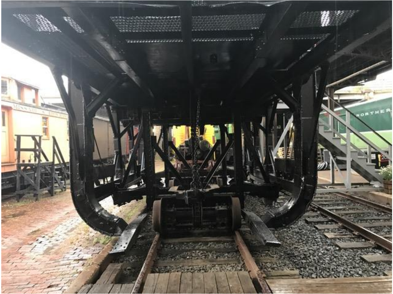
Jacks lowered outside of rails, but the wheels are not pulled for empties to pass
