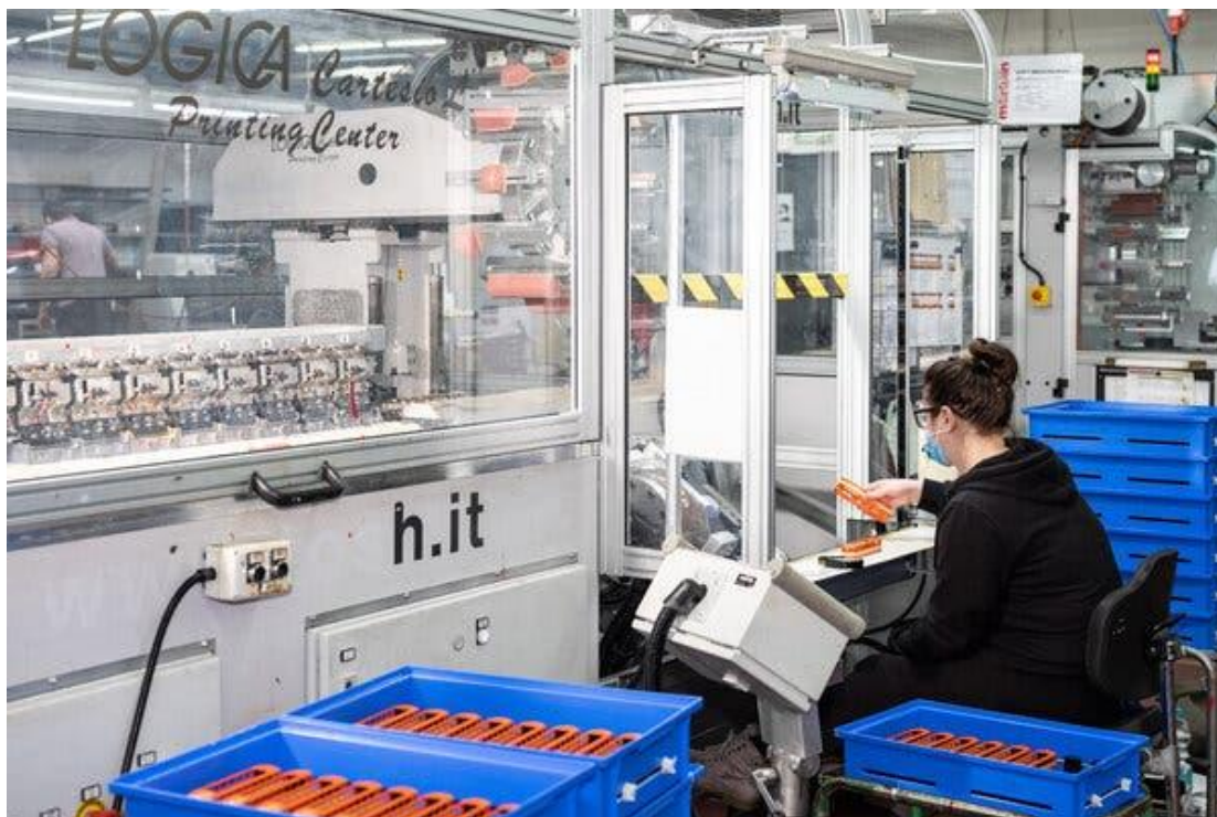
A stamp printing machine that applies detailed small prints to the casings.
