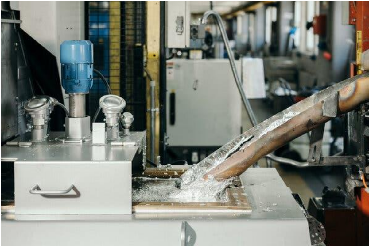
Liquid zinc alloy is filled into a tank before being cast with an industrial metal press.Credit...Felix Schmitt for The New York Times
