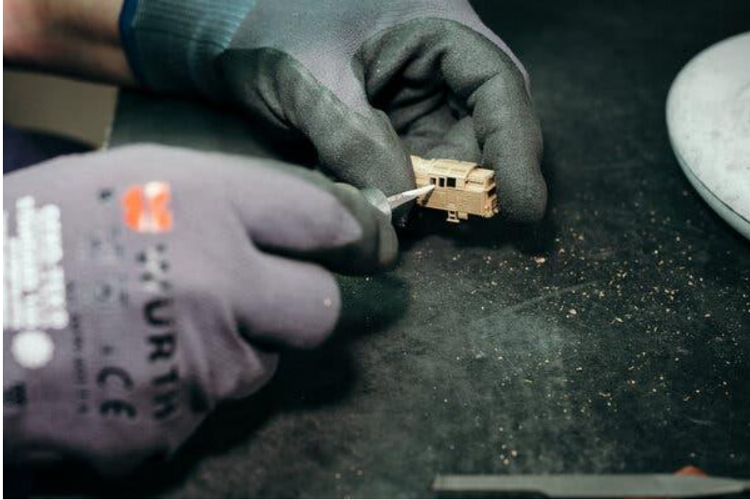
Märklin's smallest series is called Z-gauge, which is scaled at 1:220. This model train of a locomotive BR 85 is a bronze cast.
