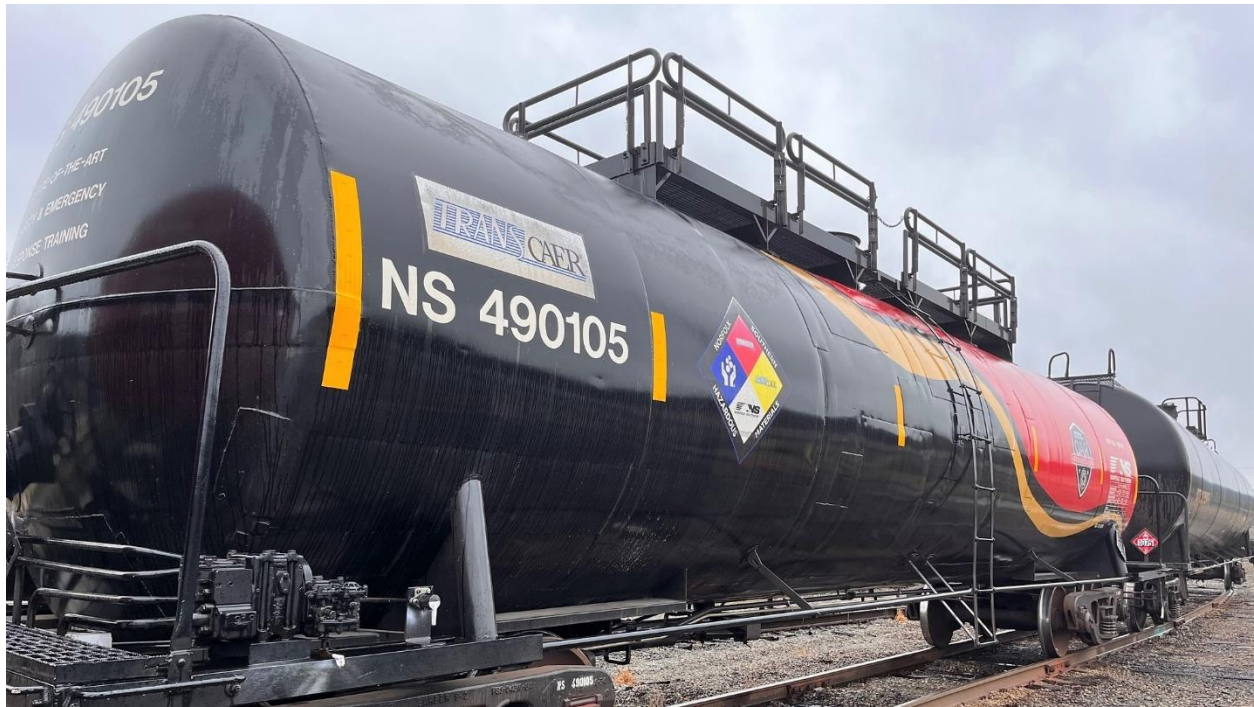
Tank car with topside training deck
