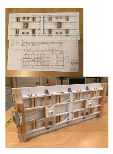
This is the completed tender chassis (rear view). Everything has been painted satin black and basswood decking planks have been added. I modified an Ozark Miniatures' link and pin coupler to accept a Kadee knuckle coupler. It turned out that the Bachmann Spectrum 0-4-0 trucks were perfect for the Mogul tender in every respect. Saved me a lot of work.
