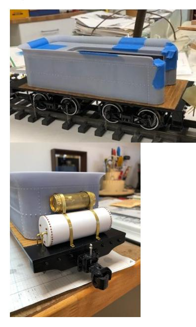
Speaking of electronics, my original goal was to make this model battery operated R/C. To make life simple down the road, I decided to mount everything on a sort of sled that could easily be removed for repairs. From left to right: the enclosed speaker, a Railboss 4 receiver on the bottom (my favorite), a brass bridge to hold the on/off and volume switches and charging jack, a Phoenix sound card, and finally the battery. Nice, neat and compact.
