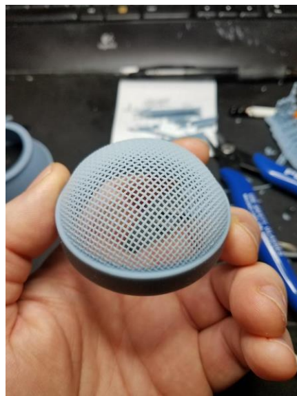
3D printed Congdon stack prototypical for this locomotive and spark arrester.
