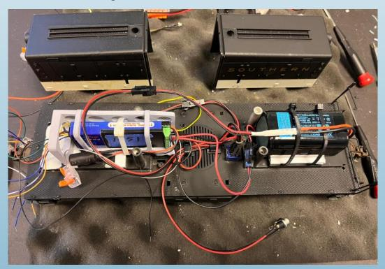
As you can see, space it tight. There are only four functions of the front and rear headlight, the cab light, and the speaker.
