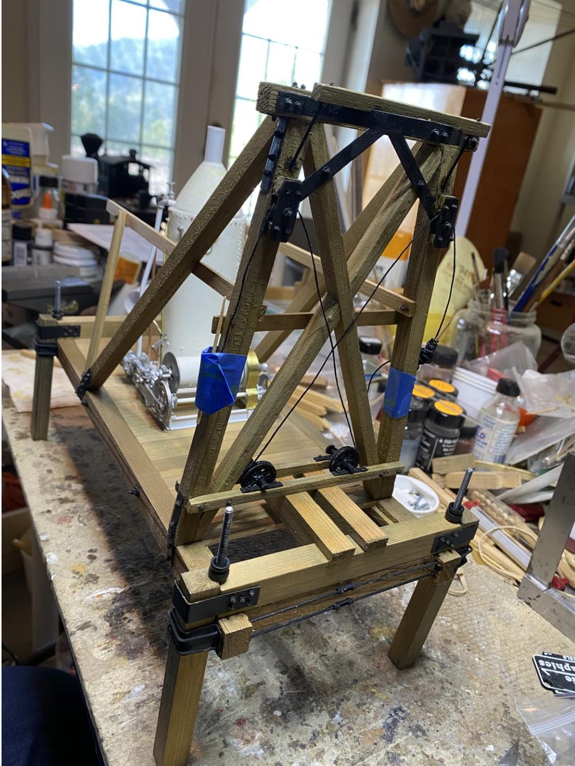
The blue tape on the mast holds the stabilizing cables out of the way. The cable is stretched out to each side to stabilize the loader after it is located at the work site.
